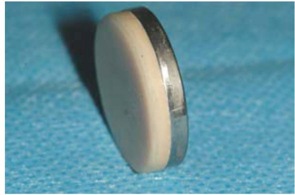
**Fig. 1** – Four different composite systems were directly bonded to Ti–6Al–4V according to the manufacturer’s guidelines.
