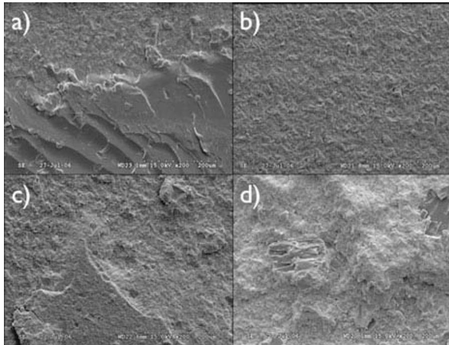
**Fig. 3 – Representative scanning electron micrographs of the metal side of fractured specimens. (a) SOL specimen presenting a mixed fracture mode; (b) Ceramage specimens presented adhesive fracture mode for all subgroups; (c) Gradia sample fractured between the opaque layer and composite; and (d) Sinfony samples presented fractures between the opaque layer and composite for all subgroups investigated.**
