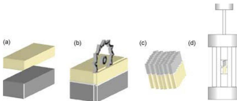
**Fig. 2** – Microtensile specimen preparation. (a) Composite system bonded to Ti–6Al–4V, (b and c) the composite-metallic substrate were reduced by means of a diamond saw under irrigation, and (d) the microtensile bars were mounted and tested in a universal testing machine.
