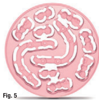
Figs. 4a & b: CAM-based milling. Fig. 5: TRINIA™ disc after milling.
