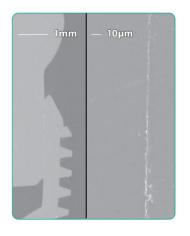
Based on a well known engineering principle, Bicon's 1.5 degree locking taper connection provides a bacterial seal at the implant to abutment interface. with a microgap of less than 0.5 microns. Bicon's bacterial seal avoids the microbial leakage issues that can result in inflammation of the soft tissue around an implant, which could lead to the loss of bone around the implant and even the loss of the implant itself. Bicon is the only system with a proven bacterial seal.
